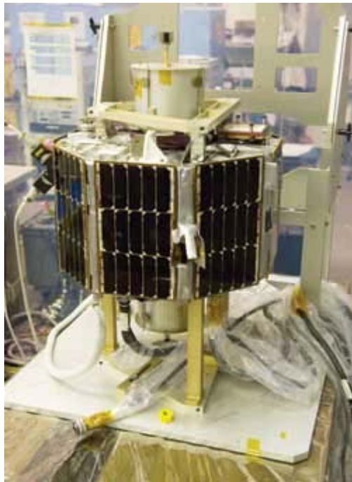
Heat management is an important concern for satellites such as the Space Technology 5 (above), launched last year. An array of MEMS-based shutters installed onboard the satellite open and close via moving microscale actuators.
