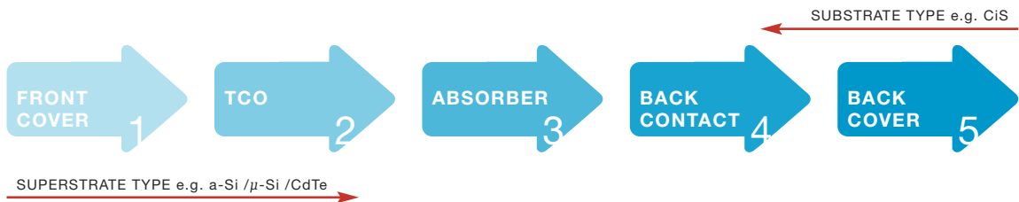
FIGURE 10 STEPS IN MAKING THIN FILM SOLAR CELLS
