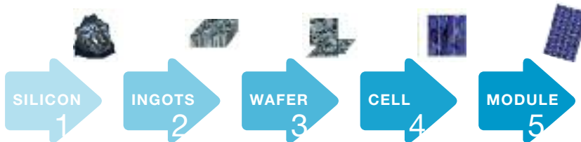
FIGURE 8 CRYSTALLINE SILICON MANUFACTURING PROCESS
