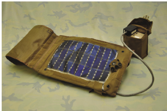
Troops in desert regions already are using MicroLink Devices' flexible, lightweight solar arrays as a source of portable, renewable energy. The panels attach to a backpack and are capable of charging military batteries, eliminating the need to carry extra ones.
