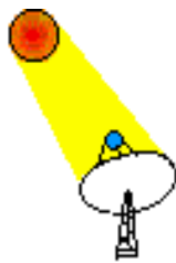
Figure 3.1 Principle of a Solar Dish (DOE II, 1997)
