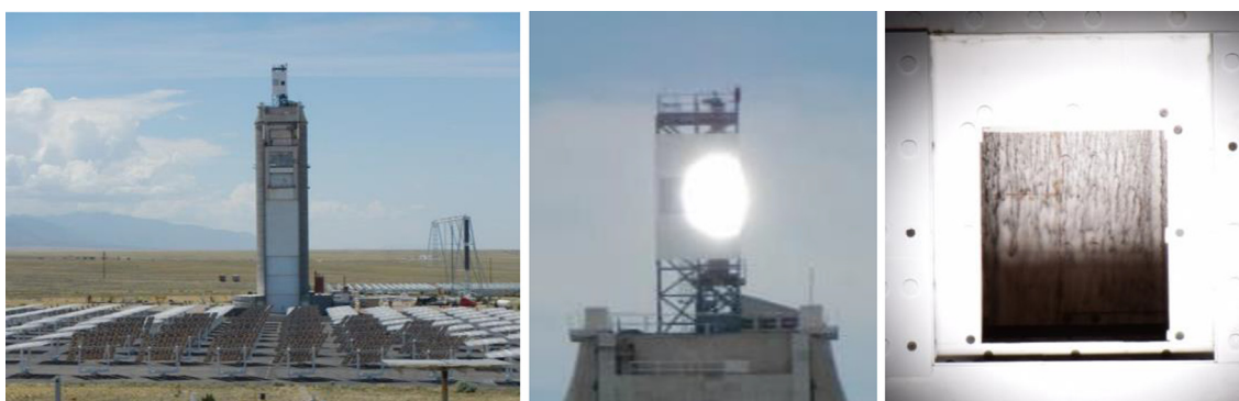
Fig. 11. On-sun testing of a falling particle receiver at the National Solar Thermal Test Facility at Sandia National Laboratories, Albuquerque, NM.
