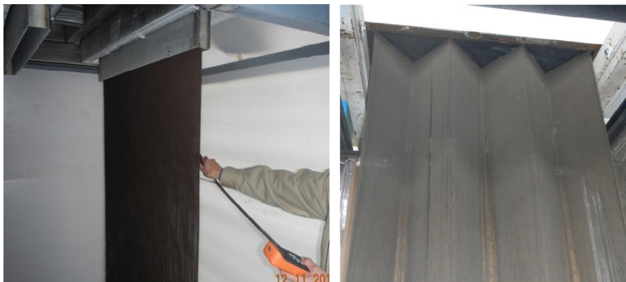
Fig. 10. Free-falling particle curtains. Alternative release patterns have been investigated to increase light trapping (Ho et al., 2016b).
