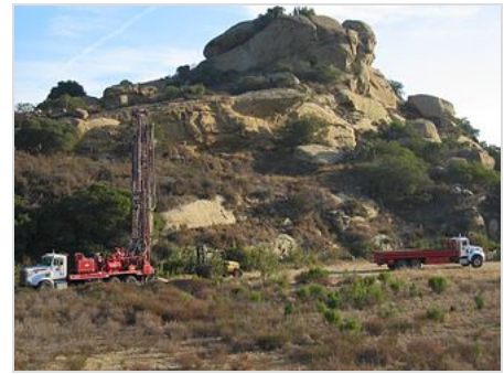
August 2004 sampling for tritium at the former Sodium Reactor Experiment facility site
