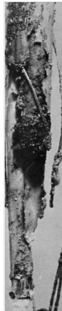
Partially melted fuel rod after the July 1959 incident
