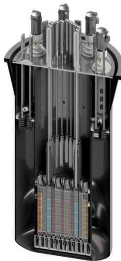
FIG. 1. Conceptual design of the Canadian Arctic SEALER [1]
