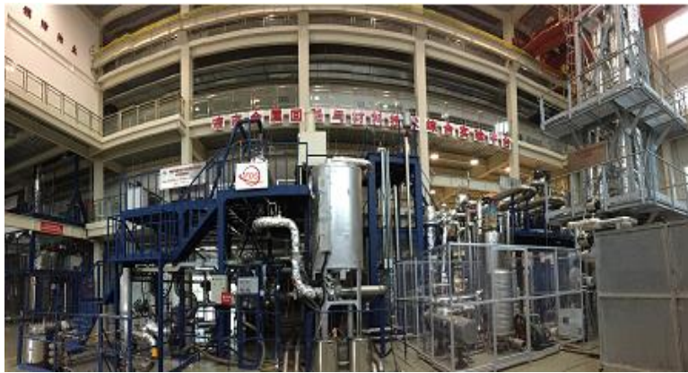
FIG. 1. Multi-functional lead-bismuth loop KYLIN-II [16]
