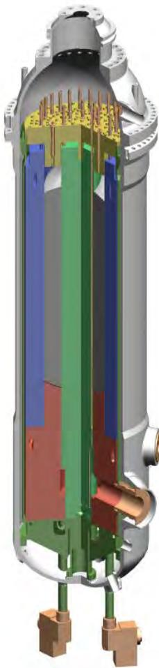
Reactor System Configuration of PBMR<sup>®</sup>-400
