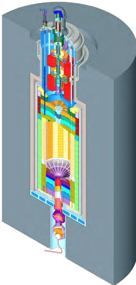
Reactor System Configuration of AHTR-100
