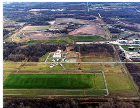
The Lake Ontario Ordnance Works (LOOW) near Niagara Falls became a principal repository for Manhattan Project waste for the Eastern United States. [346] All of the radioactive materials stored at the LOOW site—including thorium , uranium , and the world's largest concentration of radium-226 —were buried in an "Interim Waste Containment Structure" (in the foreground) in 1991. [347][348][349]
