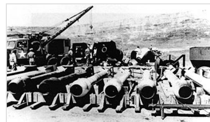
"Thin Man" plutonium gun test casings at Wendover Army Air Field, as part of Project Alberta in the Manhattan Project , illustrating their relative length and size.
