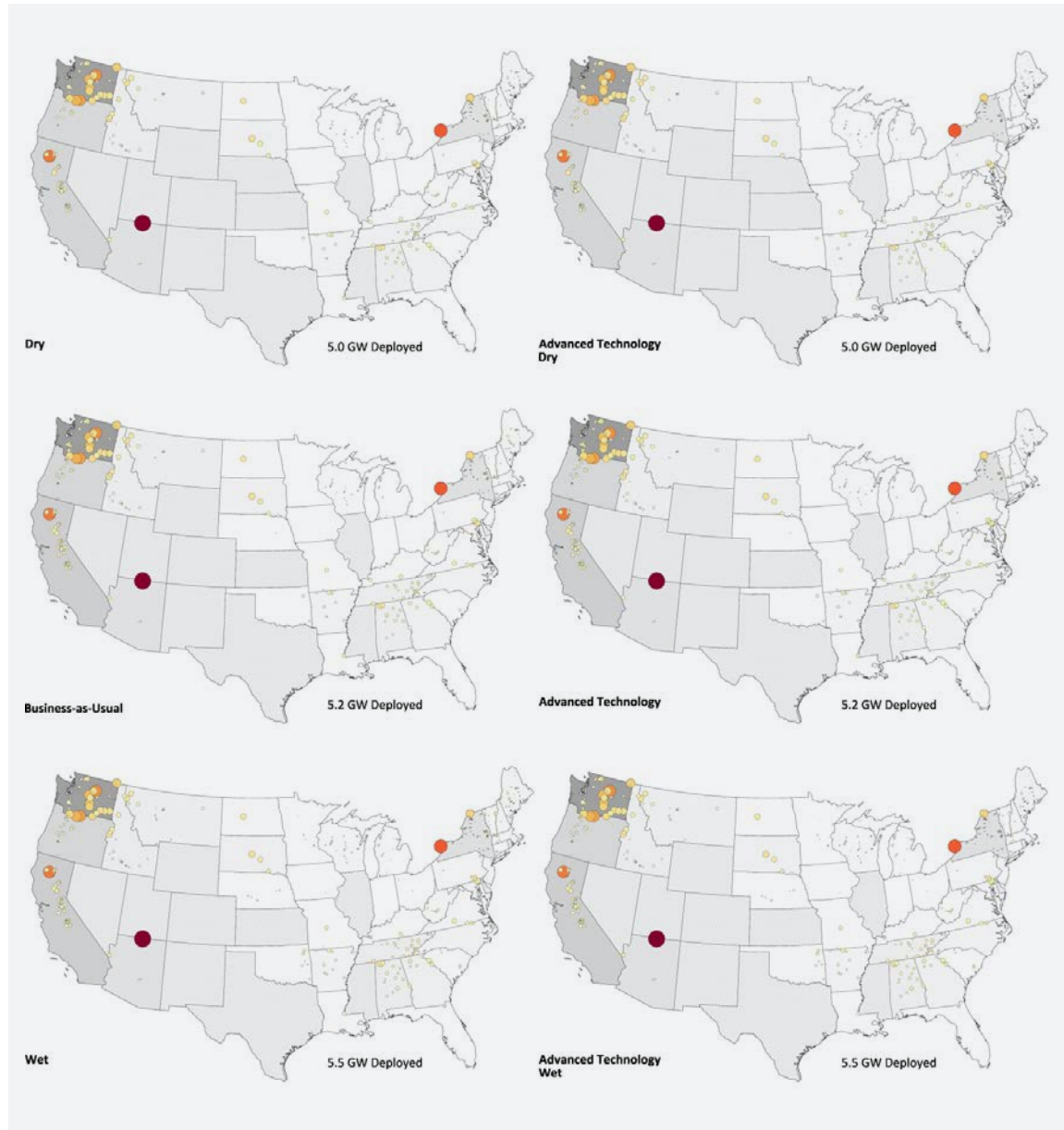
Figure F-22. National distribution of cumulative post-2016 upgrade capacity in 2050 for the Business-as-Usual and Advanced Technology scenarios and Wet and Dry sensitivities
