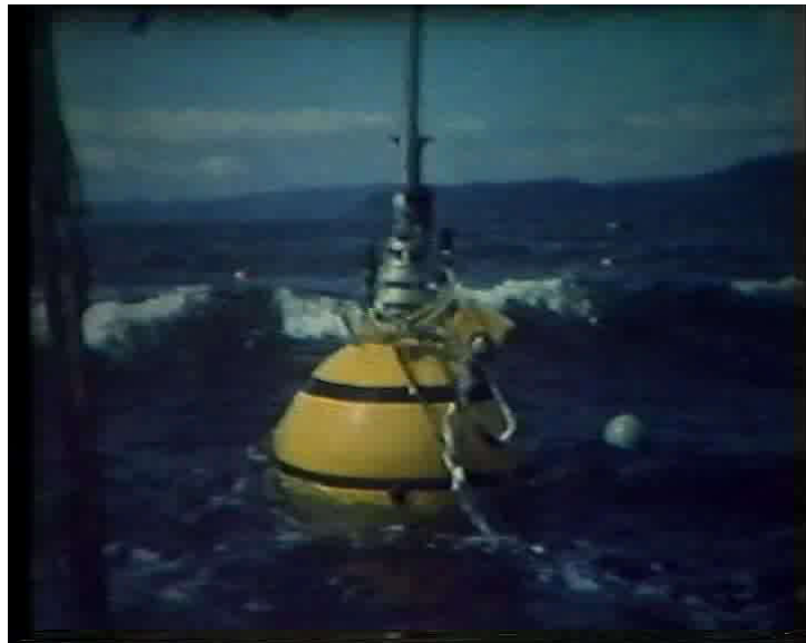
Phase-controlled power-buoy model (type E) under test in the Trondheim Fjord, 1983. Video clip [also on http://folk.ntnu.no/falnes/w_e/ .]
