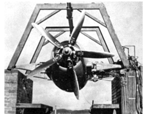
A Rolls-Royce RB.50 Trent on a test rig at Hucknall, in March 1945
