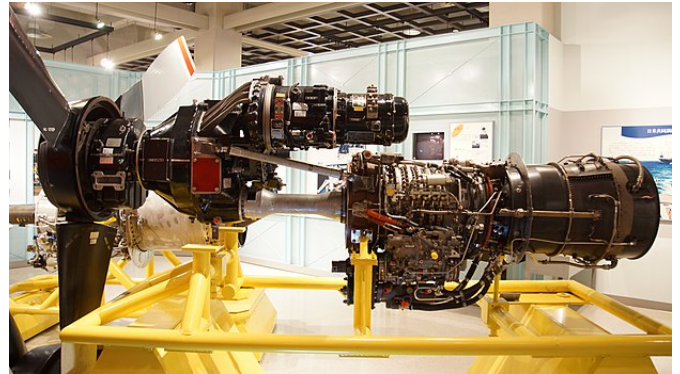
GE T64 propeller at left, gearbox with accessories in the middle, turbine core at right
