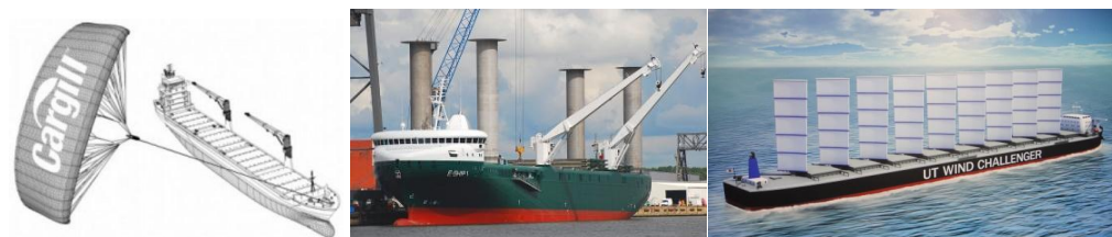
Figure 6: from left to right: Kite (Cargill, 2011), Flettner rotor (MIWB 2015) and solid sails (Wind Challenger Project HP 2015)
