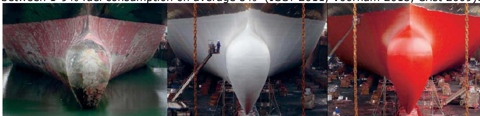
Figure 4: Example of hull coating (ECOSPEED 2015)
