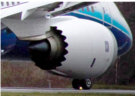
Serrated edges of the nacelle on the Rolls-Royce Trent 1000 fitted to the new Boeing 787 Dreamliner "Dreamliner".
