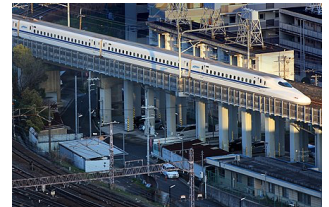
N700 Series Shinkansen uses regenerative braking
