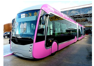
The Bus Rapid Transit of Metz uses a diesel-electric hybrid driving system, developed by Belgian Van Hool manufacturer. [79]
