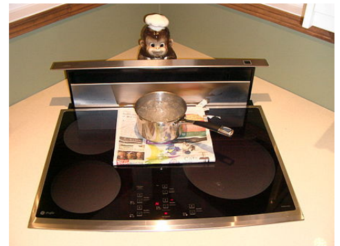
An induction cooking surface boiling water through several layers of newsprint. The paper is undamaged since heat is produced only in the bottom of the pot
