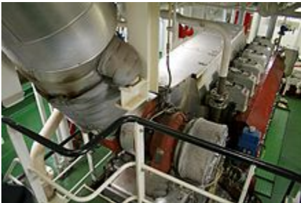
A medium-sized six-cylinder marine diesel-engine, with turbocharger and exhaust in the foreground
