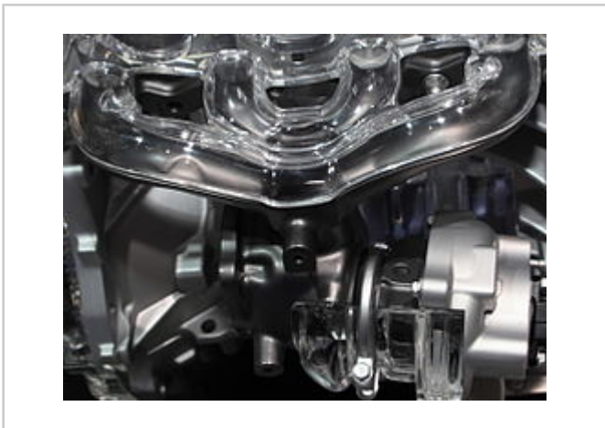
Cut-out of a twin-scroll exhaust and turbine; the dual "scrolls" pairing cylinders 1 and 4, and 2 and 3 are clearly visible
