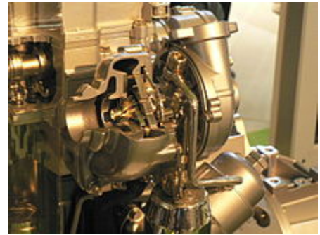
Garrett variable-geometry turbocharger on DV6TED4 engine
