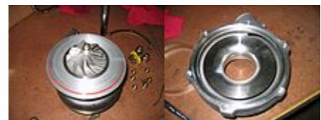
Compressor impeller side with the cover removed.
