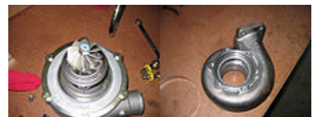
Turbine side housing removed.
