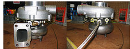
On the left, the brass oil drain connection. On the right are the braided oil supply line and water coolant line connections.
