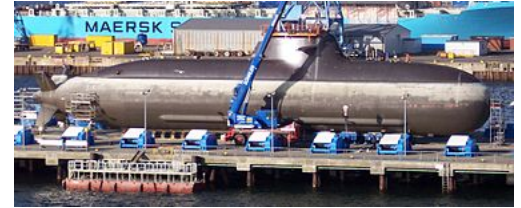
Type 212 submarine with fuel cell propulsion of the German Navy in dry dock
