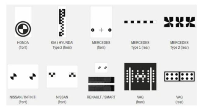
Radar targets may have patterns that appear similar to those for cameras, but include metal elements that reflect radio waves back to the sensor. Another type of radar target is a metal cone whose open end is positioned facing the vehicle to reflect radio waves back to the sensor.
