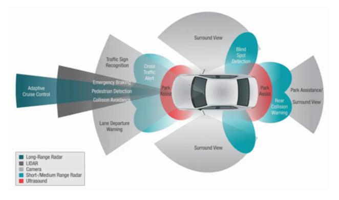
ADAS rely on inputs from a variety of sensors that allow the systems to "see" what is happening around the vehicle. The most common are camera, radar and ultrasonic sensors. Steering sensors are also used to help determine the direction of vehicle travel. While some systems use information from a single type of sensor, others combine information from multiple sensors – a process called sensor fusion – to obtain a more accurate "view" of the situation.
