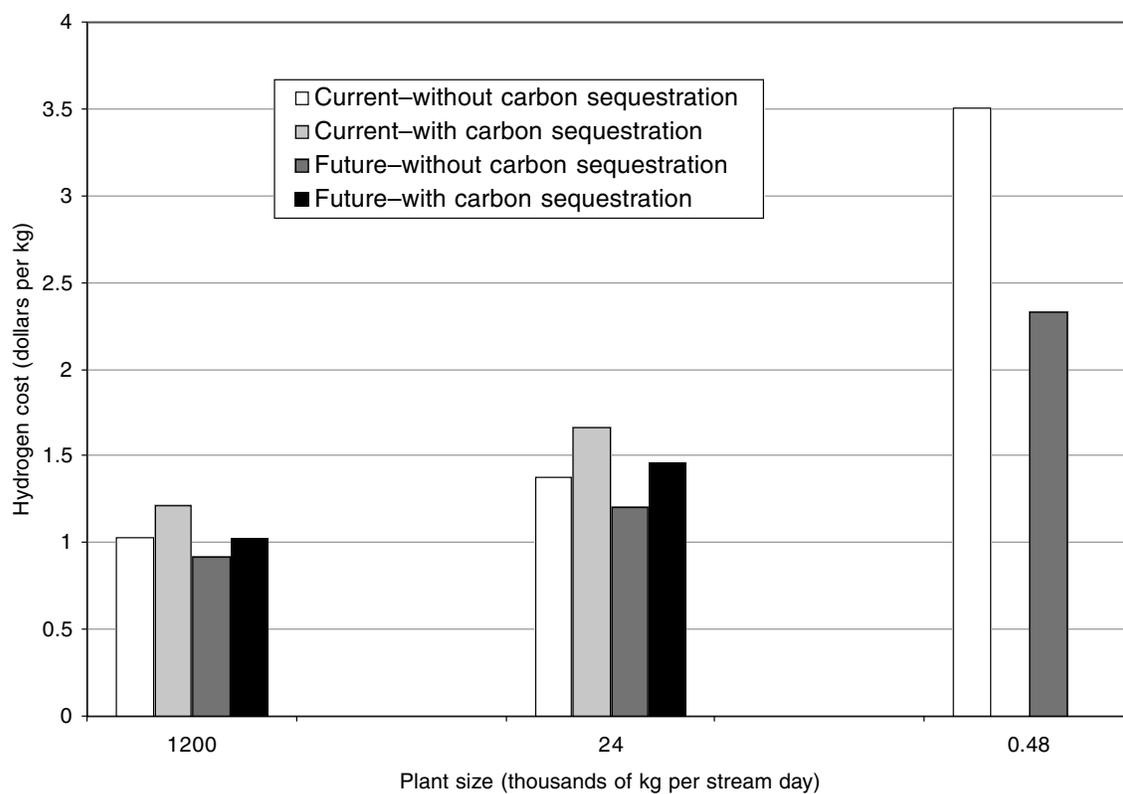
FIGURE G-3 Estimated costs for conversion of natural gas to hydrogen in plants of three sizes, current and possible future cases, with and without sequestration of CO<sub>2</sub>.
