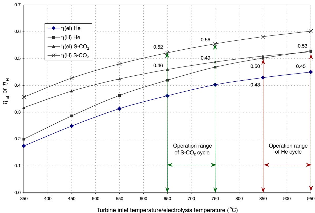
FIGURE G-5 Power cycle net efficiency ( $\eta_{el}$ ) and thermal-to-hydrogen efficiency ( $\eta_H$ ) for the gas turbine modular helium reactor (He) high-temperature electrolysis of steam (HTES) and the supercritical CO<sub>2</sub> (S-CO<sub>2</sub>) advanced gas-cooled reactor HTES technologies. SOURCE: Yildiz and Kazimi (2003).
