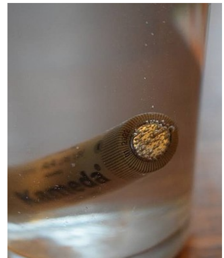
An AA battery in a glass of tap water with salt showing hydrogen produced at the negative terminal
