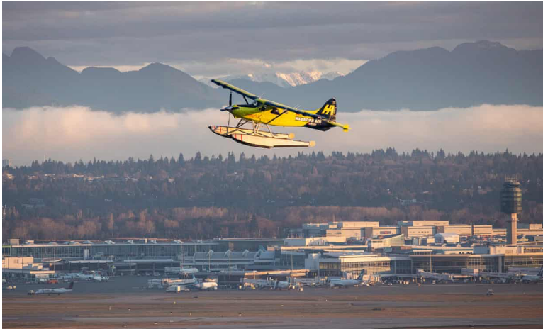
The de Havilland Canada DHC-2 Beaver, the seaplane powered by magniX that was the first all-electric commercial aircraft to fly, in December 2019. Photograph: Courtesy of Magnix
