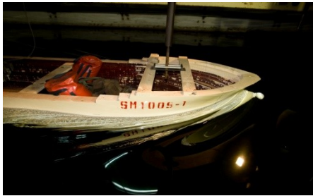
Figure 5: Design Optimisation of a 35,000dwt Bulk Carrier (A) Ship General Particulars (B) Overall Impression of Bestway Design (C) Resistance and Propulsion Model Tests (D) Hull Model For Design Optimisation
