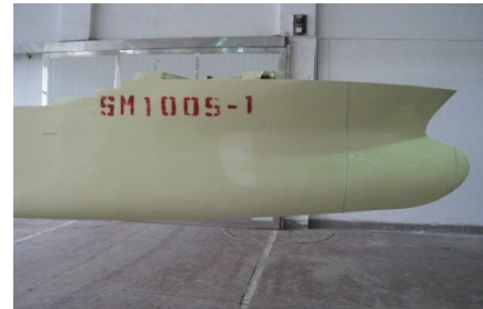
Figure 5: Design Optimisation of a 35,000dwt Bulk Carrier (A) Ship General Particulars (B) Overall Impression of Bestway Design (C) Resistance and Propulsion Model Tests (D) Hull Model For Design Optimisation
