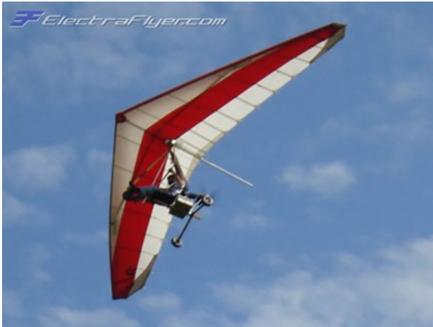
ElectraFlyer Trike electrically powered microlight. (ElectraFlyer.com)
