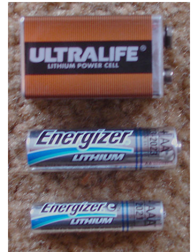
Lithium 9 volt, AA, and AAA sizes. The top object is a battery of three lithium-manganese dioxide cells, the bottom two are lithium-iron disulfide cells and are compatible with 1.5 volt alkaline cells.
