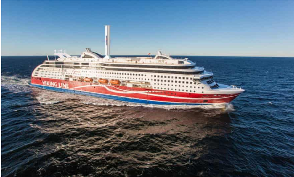
LNG-powered Viking Grace boasts the first ship-based 'rotor sail'. Photograph: Tuukka Ervasti/Lloyd's Register
